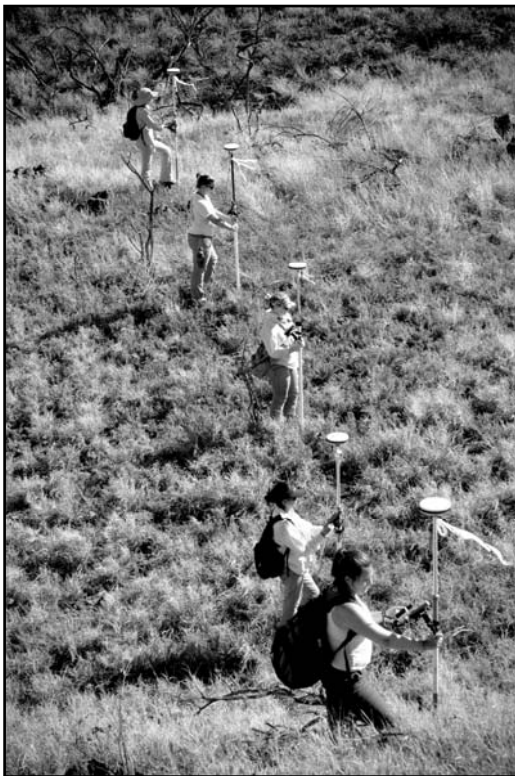
Figure 2 - Micro-topographic Survey Transect. Surveyors shown here with roving GPS unit and an antenna on a survey rod.
